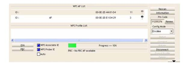
Users can click 'PBC' button few more times to try again. When an access point is connected, users can click 'Disconnect' to disconnect your wireless network card from a connected access point. Users can also click 'Rotate' button, and next access point on the list will be selected to establish connection.
